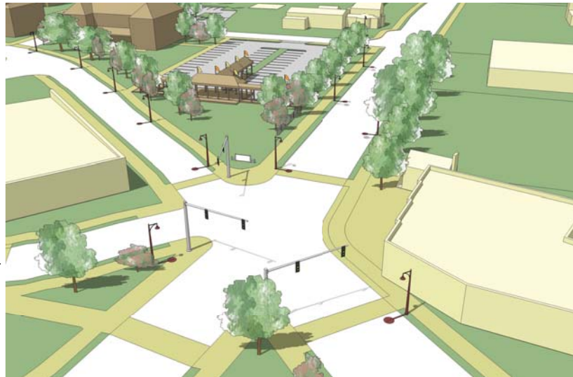
Using a GIS base map of the town, this 3-D rendering of Warsaw was made with SketchUp software to help the community visualize proposed improvements.
