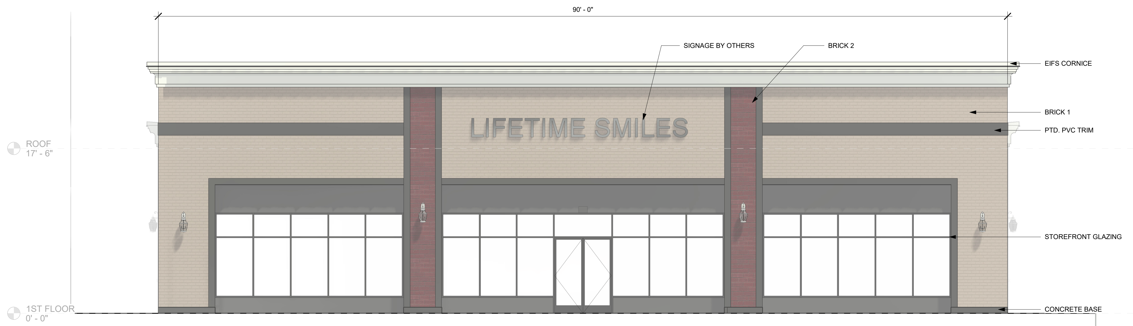
3 ARB - FRONT ELEVATION - BRICK ON 3 SIDES 3/16" = 1'-0"
