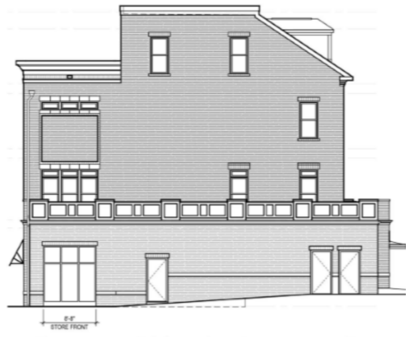
4 A-100 SCALE: 1/8" = 1'-0" BUILDING 'A' - RIGHT SIDE ELEVATION
