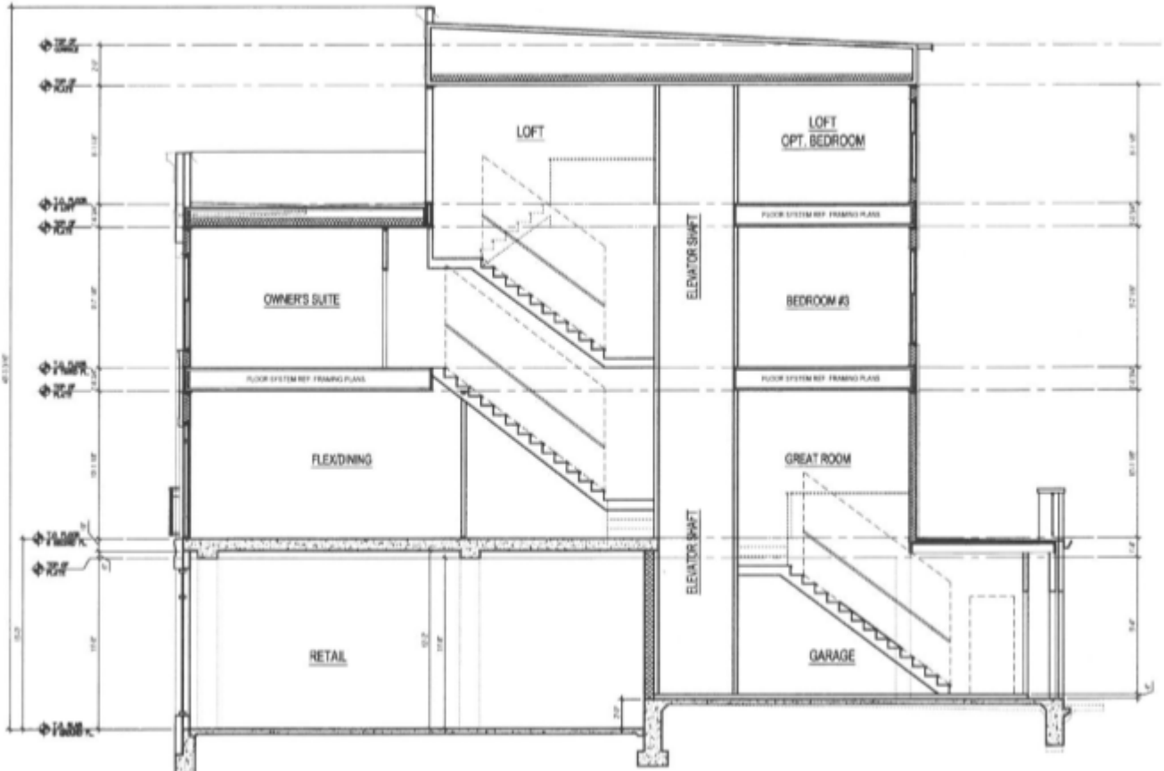
BUILDING 'B' SECTION SCALE: 1/4" = 1'-0" DATE: 11/15/19
